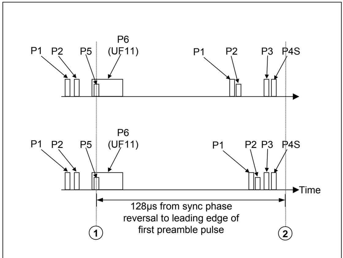
**Figure 9. Combination of Mode S and Mode A/C in Same All-Call Period**
