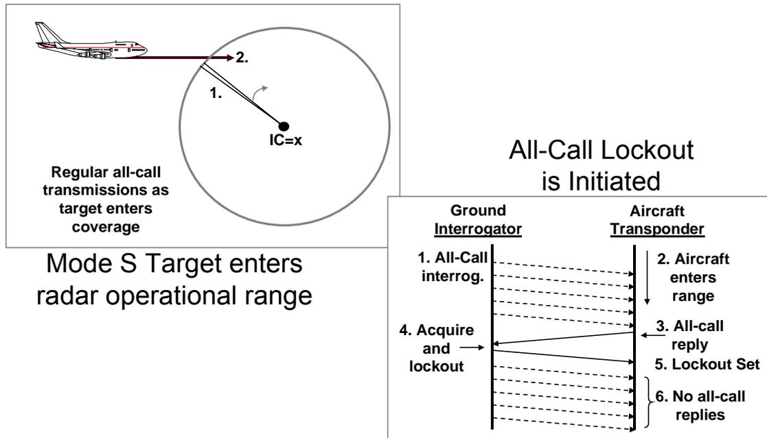
**Figure 2. Stages of Lockout**
