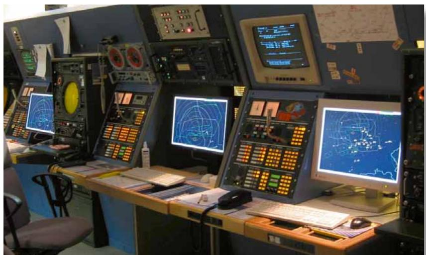
**Radar Approach Control at a German Air Force Base using CIMACT**
