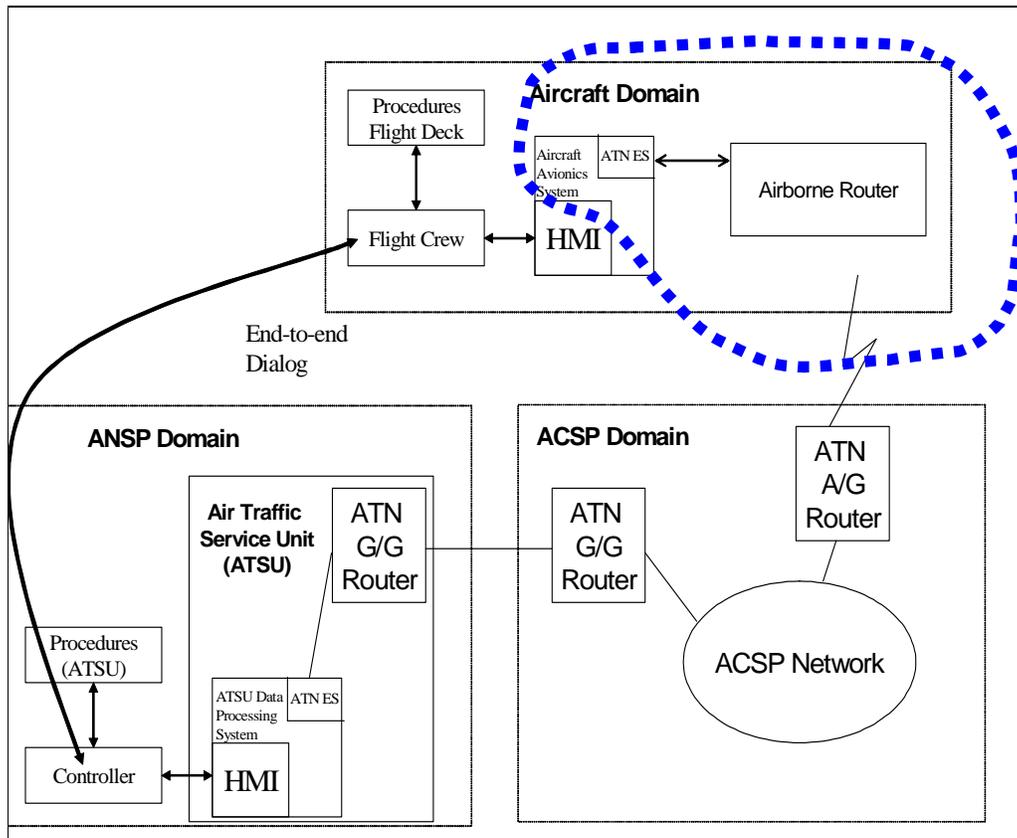
Figure 1- ATN Data Link System Functional Architecture
