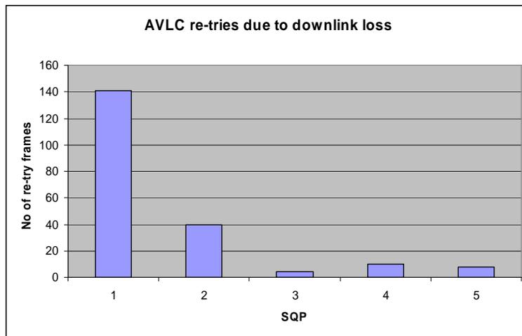
This figure illustrates that there is a substantially higher risk of AVLC re-try due to downlink loss at SQPs less than 2. The losses at SQP 0 are not shown because generally aircraft had initiated handoff to another VGS before recording significant AVLC re-tries at this level.
