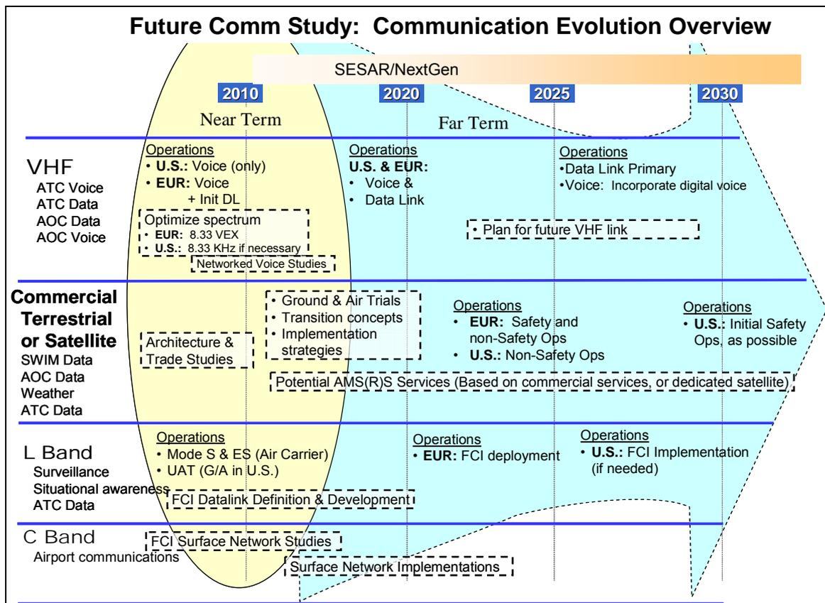
Figure 1 Aeronautical Mobile Communications Evolution Overview
