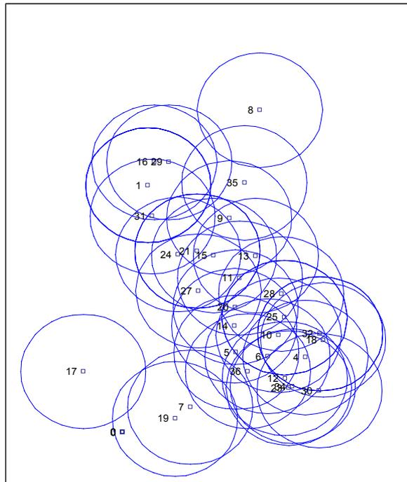
Figure A-12 - Coverage of a typical set of VHF radio stations (107NM – FL100)
