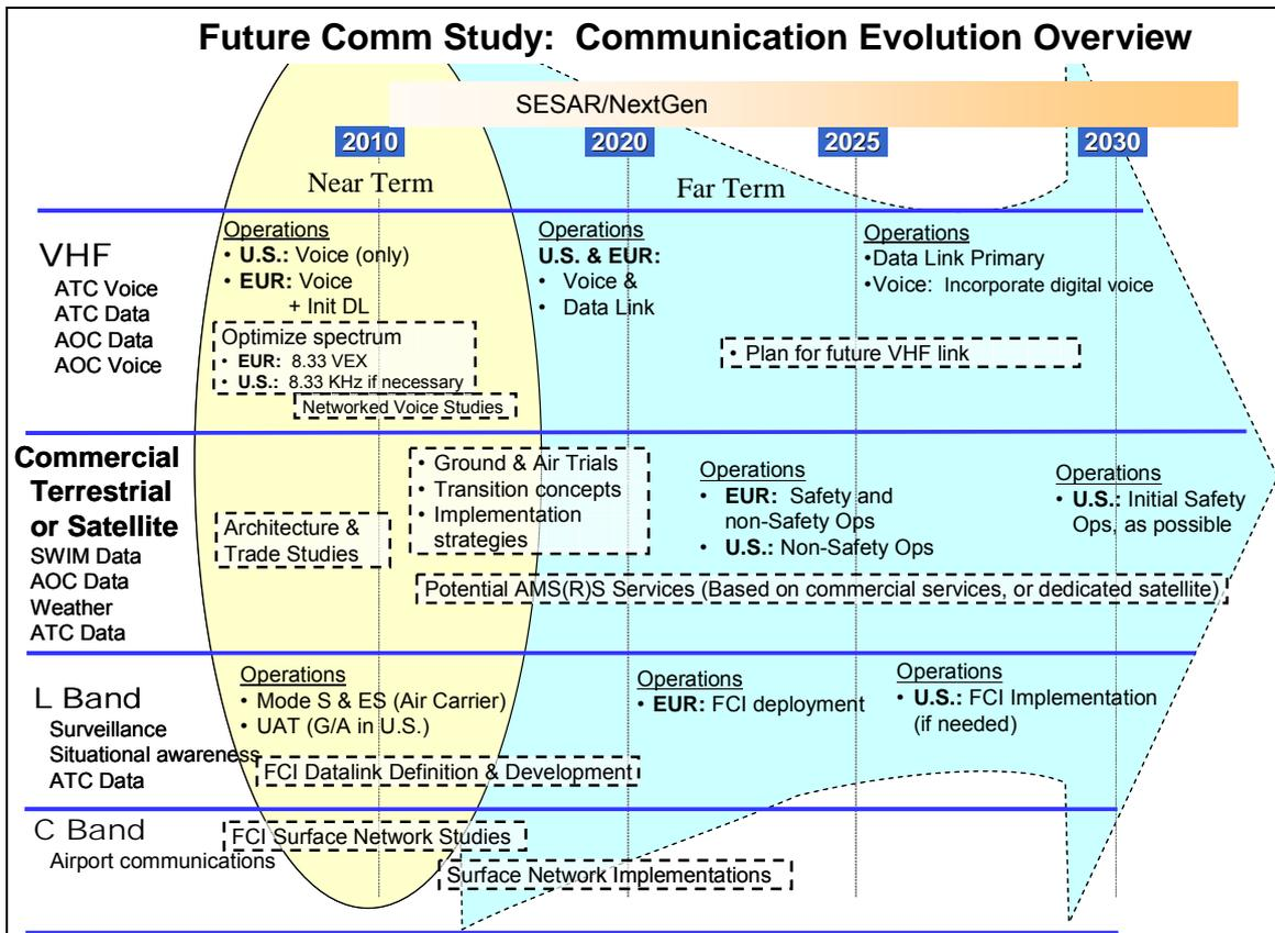
**Figure 3 – Aeronautical Mobile Communications Evolution Overview**
