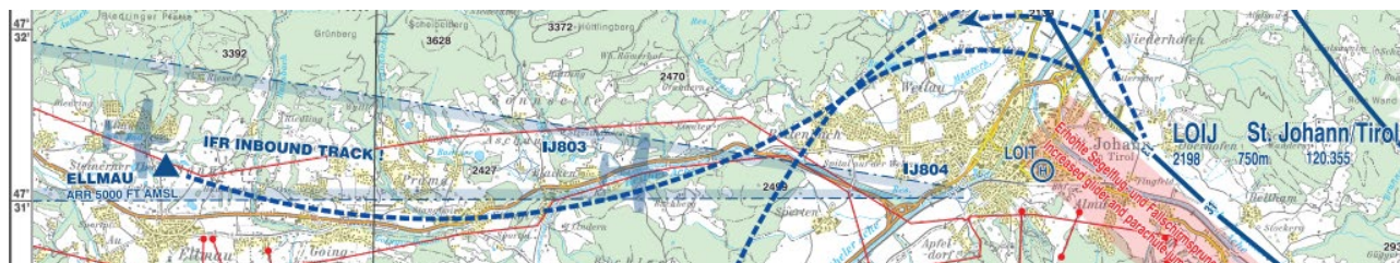
IFR approach sector representation on the VFR chart [source: AustroControl Chart for VFR flights ST. JOHANN/TIROL]
