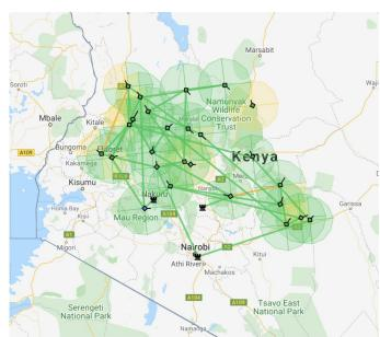
A network of 25 interconnected, continuously moving, automated HAPS delivering internet in Kenya in July 2020. Altitude: FL500 - FL620 - Operations managed from multiple locations: London, UK - California, USA, Michigan USA
