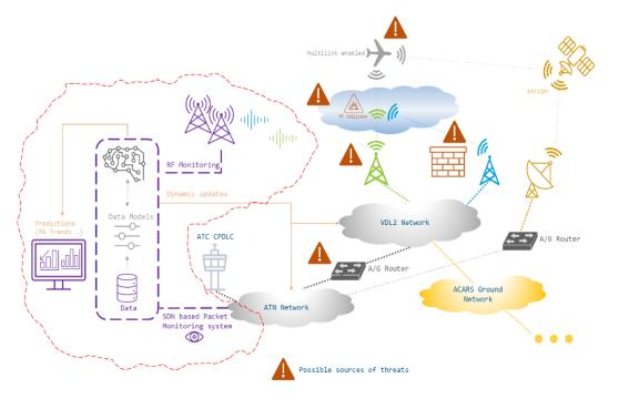
Software defined networking architecture augmented with Artificial Intelligence to improve aeronautical communications performance, security and efficiency
