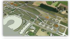
**RELs** that are **ON** (illuminated red) indicate that the runway ahead is not safe to enter or cross. THLs that are **ON** (illuminated red) indicate that the runway is not safe for takeoff. RED MEANS STOP! Pilots should remain clear of a runway when an REL along their taxi route is illuminated. Pilots should not takeoff when a THL on the runway ahead is illuminated.
