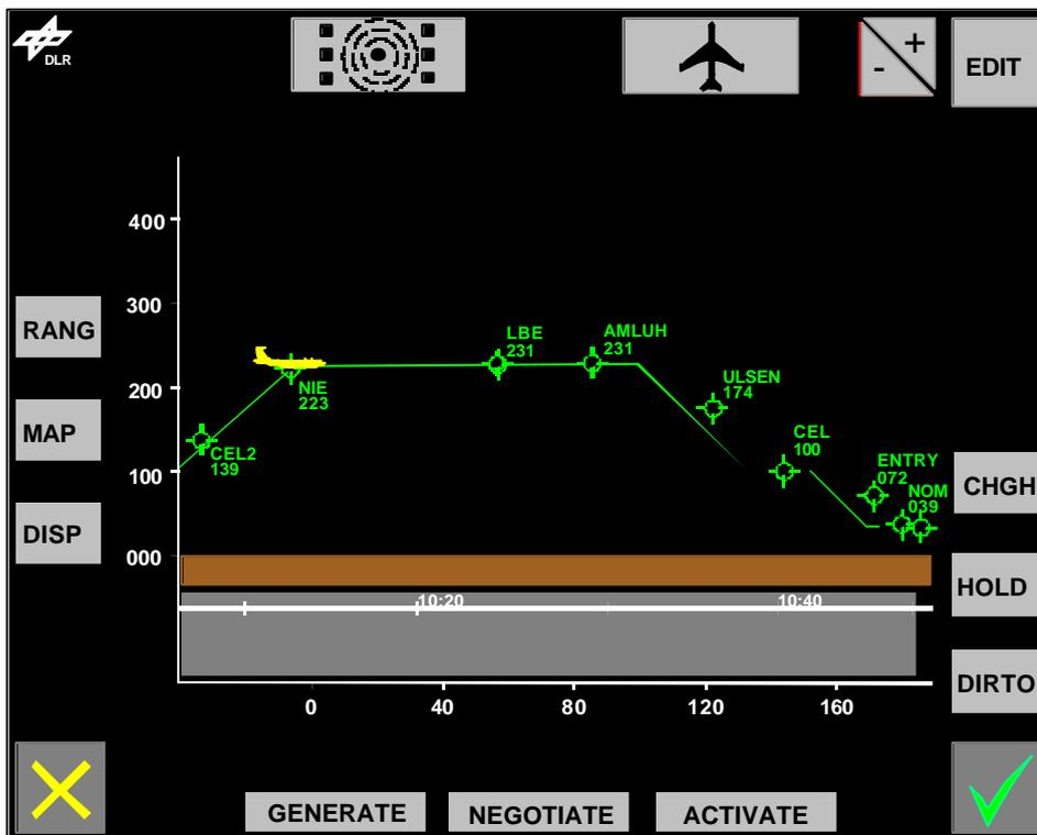
Figure 2.5 ND - Vertical Display, MONITOR Mode
