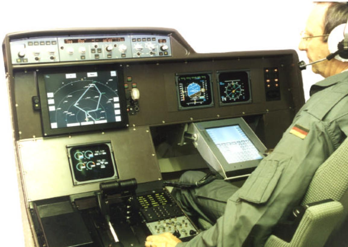
*Figure 1.2 ATTAS Experimental Cockpit with CDU and AHMI Display*
