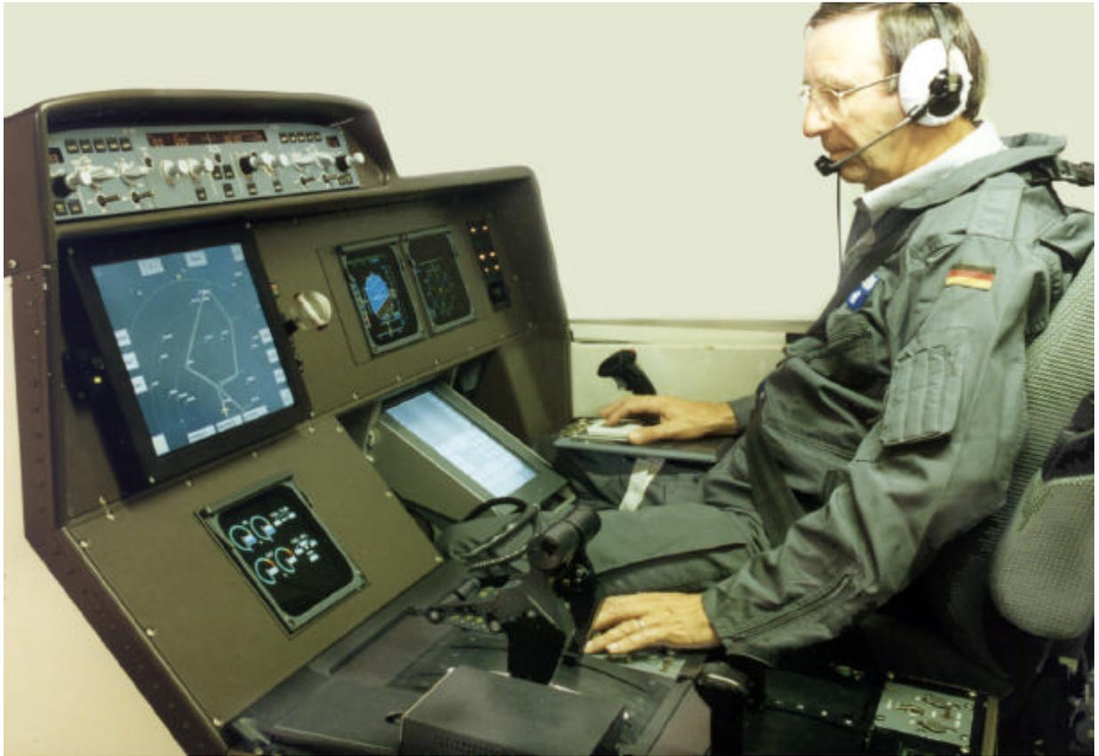
*Figure 2.1*      *ATTAS Experimental Cockpit with Pilot operating the Touch-pad Input Device (with his right hand)*
