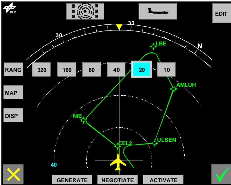
Figure 2.4 ND - Horizontal Display, MONITOR Mode, RANGE Select Sub-Menu activated
