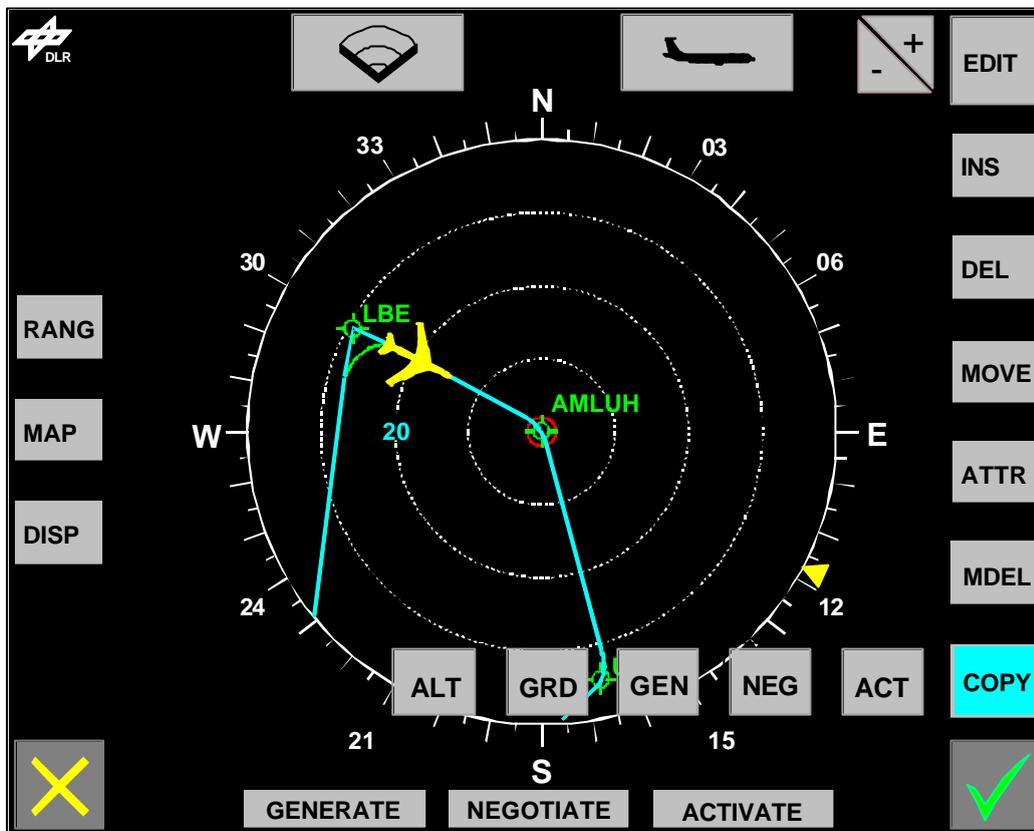
Figure 2.6 Bottom Part of ND in PLAN Mode with COPY Sub-Menu opened
