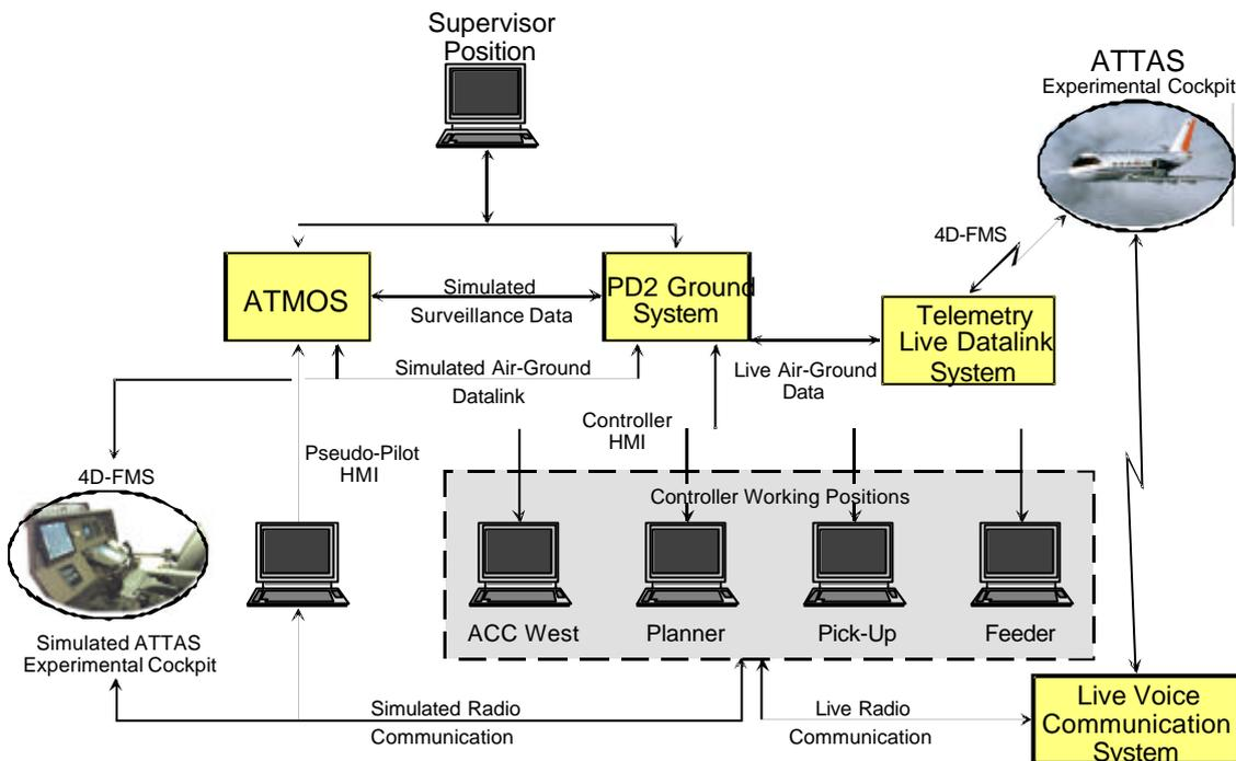
Figure 3.1 PD/2 Trials Configuration incorporating ATTAS and ATTAS Flight Simulator
