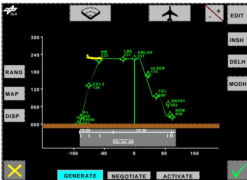
Figure 2.3 ND - Vertical Display, PLAN Mode
