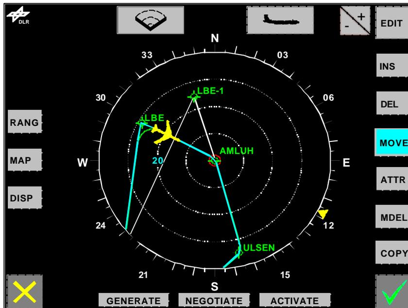
Figure 2.2 ND - Horizontal Display, PLAN Mode
