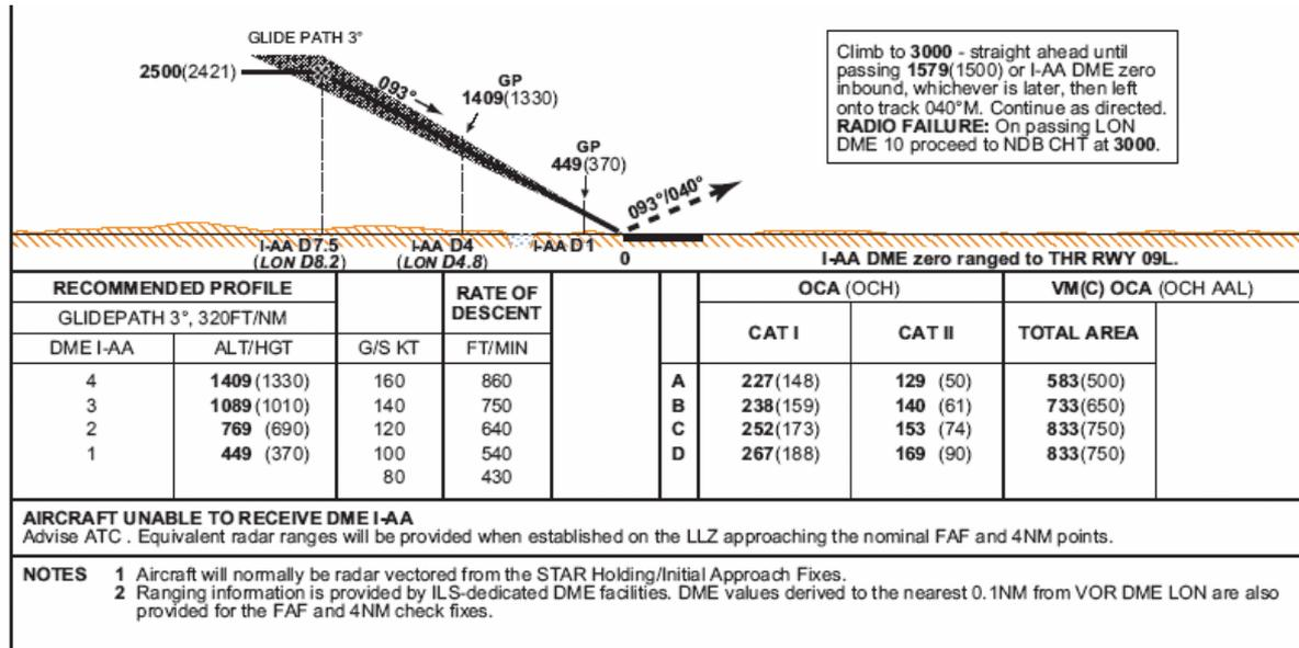
Note small level segment at 2500ft prior to joining ILS, which ends at the Final Approach Fix. Referred to in procedural approach instructions in AIP.
