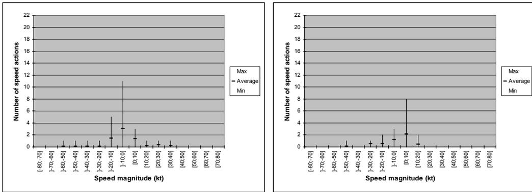
Figure 32: Distribution of speed actions magnitude in the “acquisition” phase of the large (left) and small (right) initial spacing deviation condition.
