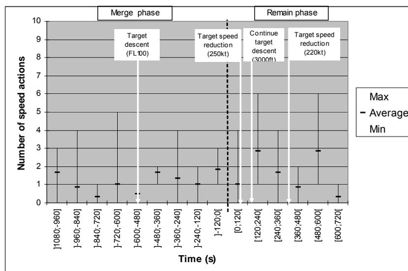
Figure 23: Temporal distribution of speed actions for a LFPG scenario with a small initial spacing deviation.
