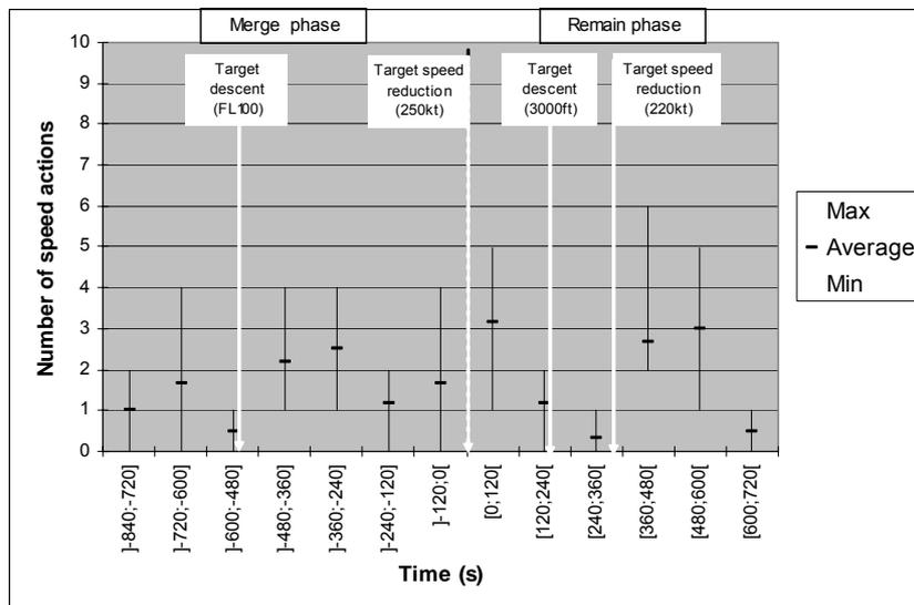
Figure 25: Temporal distribution of speed actions for a LFPG scenario with a large initial spacing deviation.
