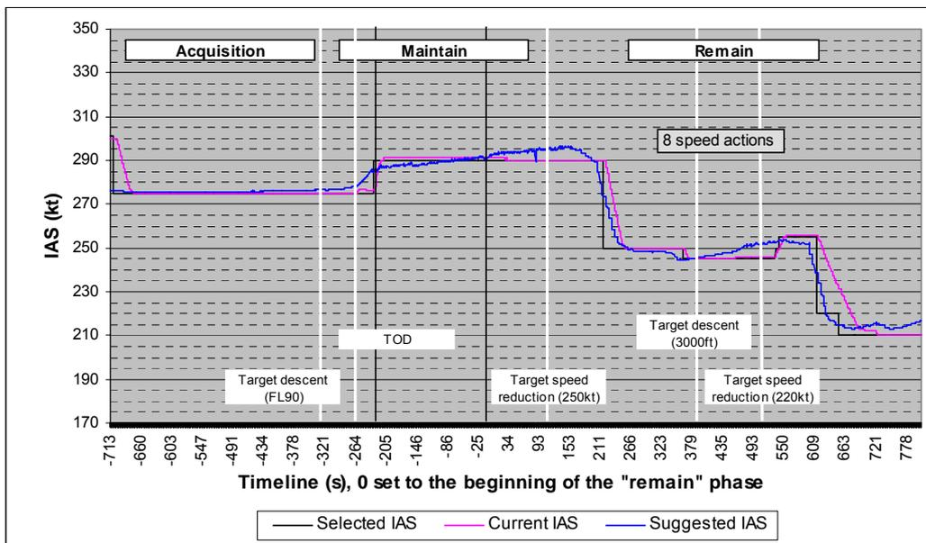
Figure 17: Example of a speed profile for a LFPO scenario with a large initial spacing deviation.
