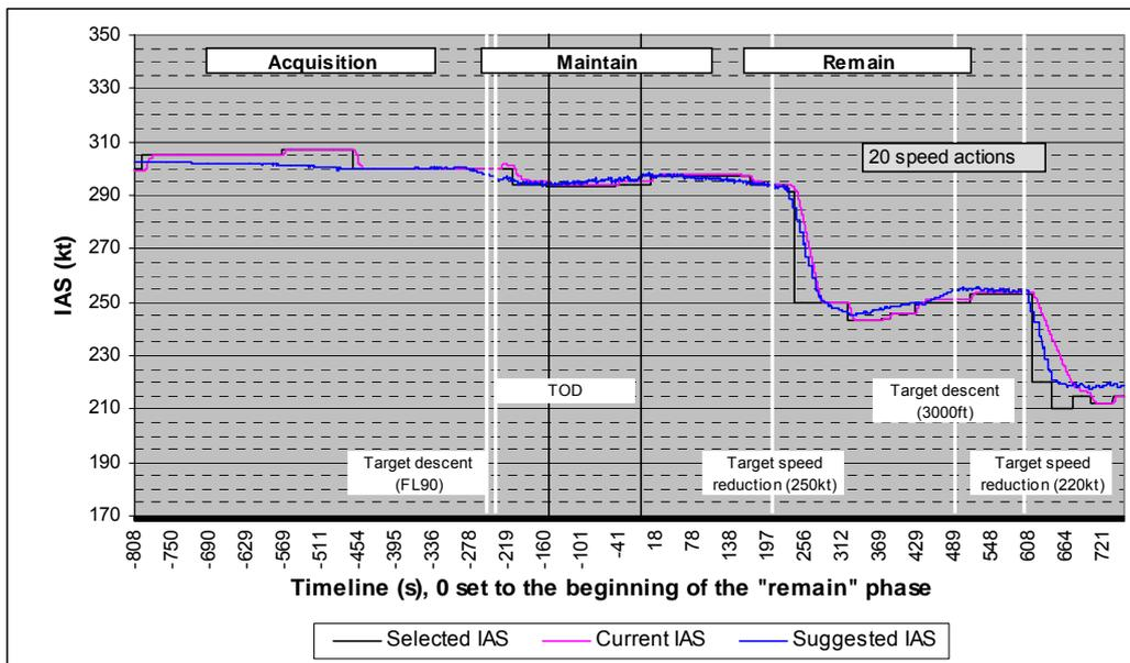
Figure 15: Example of a speed profile for a LFPO scenario with a small initial spacing deviation.
