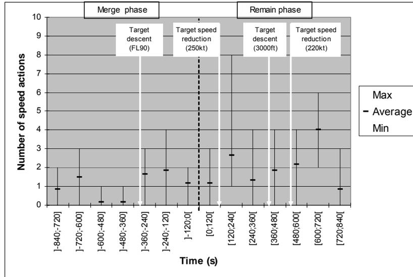
Figure 24: Temporal distribution of speed actions for a LFPO scenario with a small initial spacing deviation.
