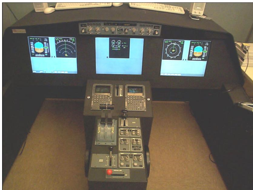
Figure 5: Cockpit Simulator.
