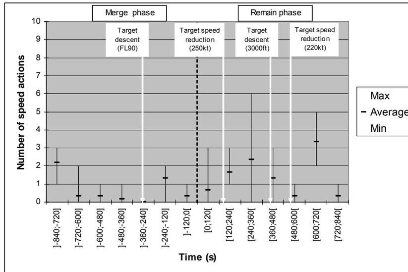
Figure 26: Temporal distribution of speed actions for a LFPO scenario with a large initial spacing deviation.
