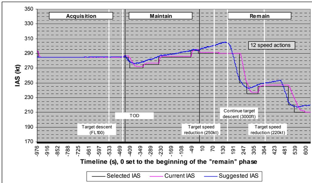
Figure 14: Example of a speed profile for a LFPG scenario with a small initial spacing deviation.
