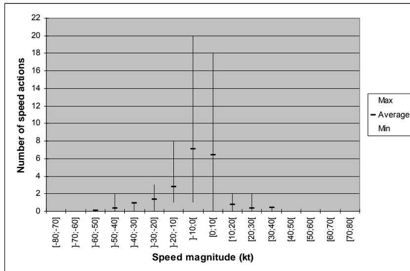
Figure 31: Distribution of speed actions magnitude in the small initial spacing deviation condition.
