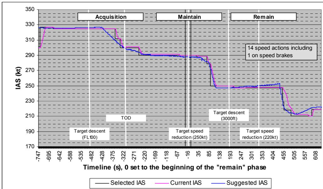
Figure 16: Example of a speed profile for a LFPG scenario with a large initial spacing deviation.
