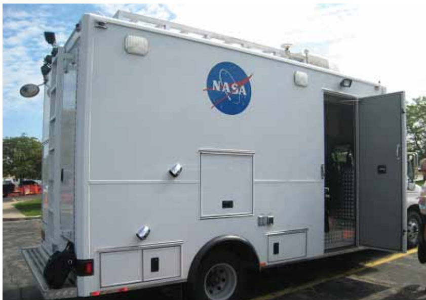
Figure 4 – NASA Glenn's Aeronautical Research Vehicle (ARV) equipped to perform AeroMACS mobility testing and demonstrations.
