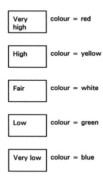
Every two minutes the controller will be prompted to press one of these buttons according to their assessment of workload at that point. The requirement to do this will be indicated by the red light on the ISA box becoming illuminated. The prompt will remain illuminated for a fixed period of time (or until the controller makes his selection) after which no selection will be accepted. This time period can be varied but is currently set at 30 seconds.
