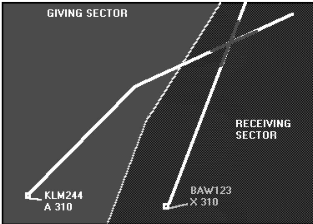
*Fig iv. Test 2; pass - BAW123 is not known to the giving sector.*
