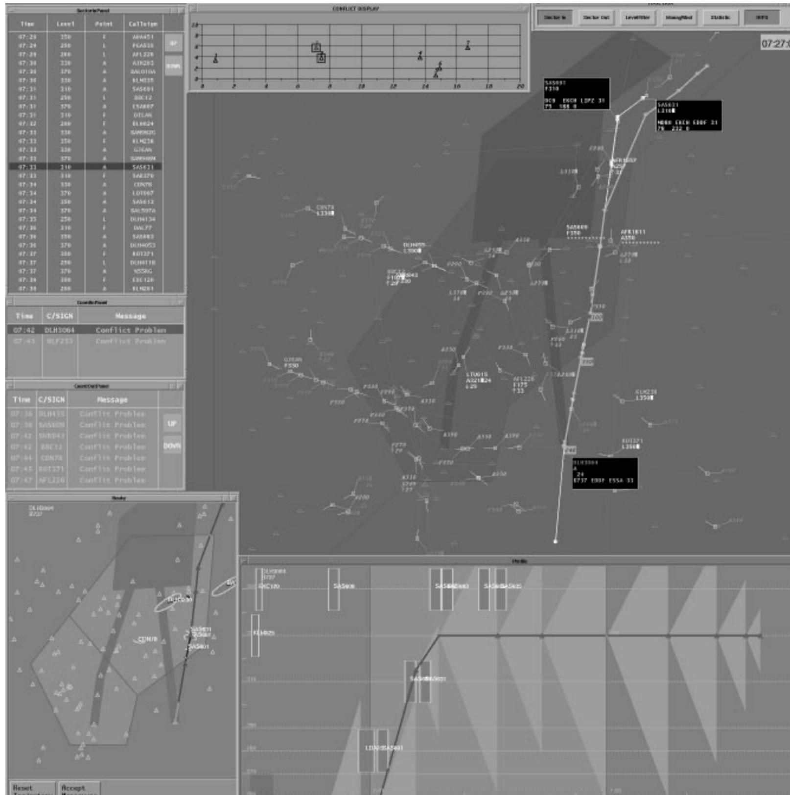
The HIPS has been activated to examine a conflict on the trajectory being requested by DLH3064 just airborne from Frankfurt north bound. The Flight Leg of the DLH is green to show that this is the plan that is on view in HIPS, it is the 'subject' aircraft.
