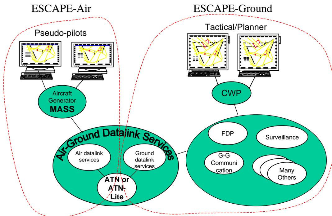
Figure 3: Functional Overview of ESCAPE Simulator
