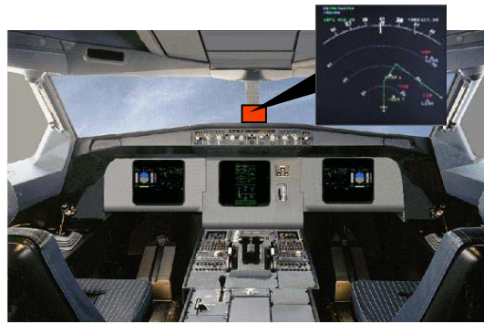
Figure 1 - On board equipments supporting ASAS (at the center of the cockpit simulator)
